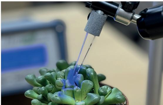
For measuring smaller samples such as Arabidopsis, needles and lichens, two tapered light guides are available. The tapered form of these light guides focuses the light from FMS-300 and increases the maximum saturating pulse intensities. The two light guides have dimensions at the sample end of 4 x 4 mm and 2.5 x 2.5 mm providing up to 60,000 and 90,000  $\mu\text{mol m}^{-2} \text{s}^{-1}$  respectively.
